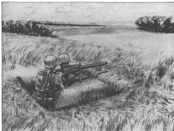
FIGURE 66. —Caliber .30 machine-gun (light) emplacement, open standing type.
