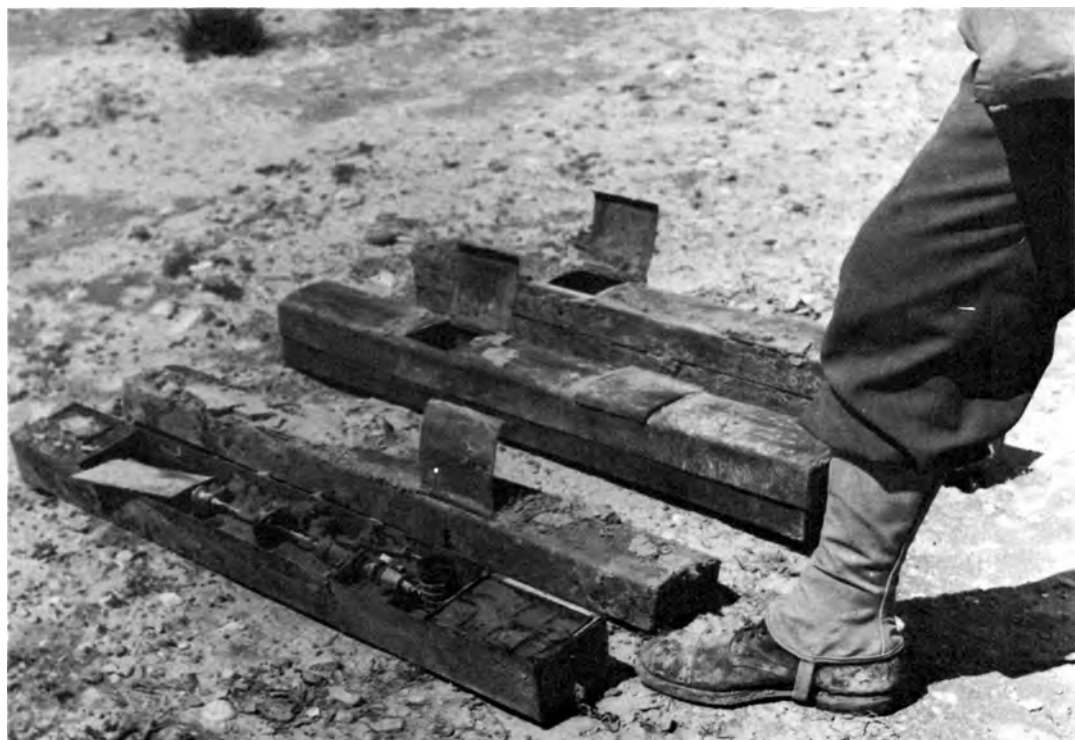
ITALIAN BAR MINES. The opened casing shows the simple pressure detonating device.
